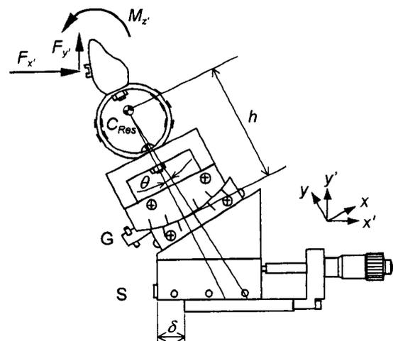
Figure 2. Orthodontic simulator with tooth root designed as a ring sensor.
