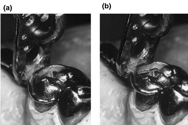
**Fig. 9.** (a) An experimental view from a motion picture of a framework A in its early dislodgment stage in the suspension test before the load (retentive force) reached the peak. (b) Another view of the same framework immediately after the peak load was recorded. Note that the framework with the retention plate lingually rotated.
