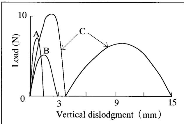
Fig. 7. Load-vertical displacement curves of representative frameworks each from the three designs (A, B, and C) in the suspension test.
