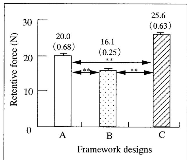
**Fig. 6.** The means and standard deviations of the retentive forces for the three designs in the grip test.
