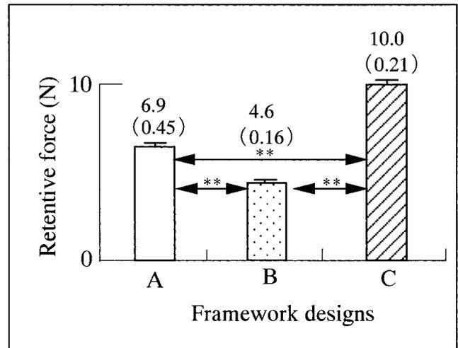
Fig. 8. The means and standard deviations of the retentive forces for the three designs in the suspension test.
