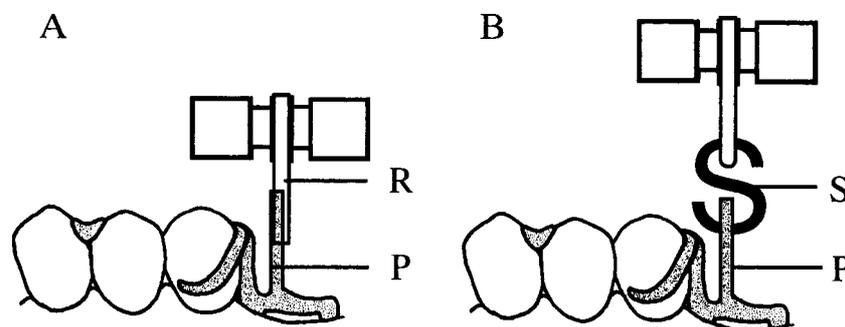
**Fig. 4.** Schematic illustrations of the dislodgment test. A, grip test; B, suspension test; P, retention plate in the framework saddle; R, tensile rod connected to the universal testing machine; and S, S-shaped metal hook.
