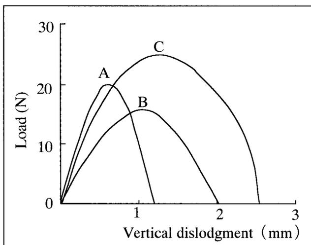
**Fig. 5.** Load-vertical displacement curves of representative frameworks each from the three designs (A, B, and C) in the grip test.
