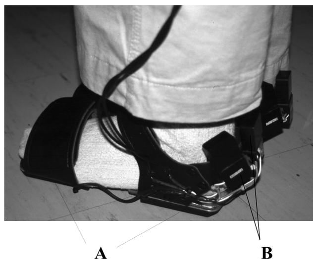
**Fig. 1.** Shoes of the measuring devices. A: strain gauges attached on the heels and toes of the shoes; B: transmitters attached to the shoes.
