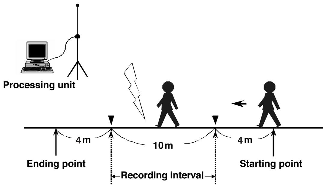
**Fig. 2.** Scheme of the gait measurements. The electrical signals, which were detected by the strain gauges attached to the shoes, were transmitted to the processing unit. The midst 10m-walk was taken for analysis.
